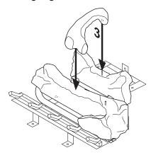
Figure 47 - Installing Log No. 3
